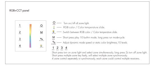
Note: After touch power key to turn off light, long press power key for 5 seconds will turn on or turn off tone.
